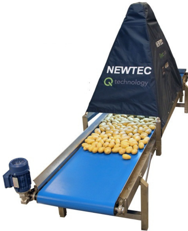
Figure 10.6.: Newtec SCOUT - 3D Sensor Camera
