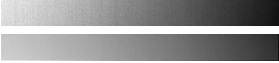
Figure 7.2.: Fixed Pattern Noise due to column amplifiers
