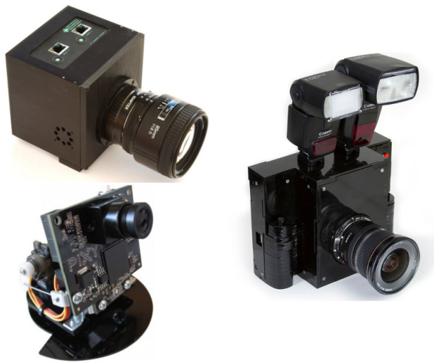
Figure 2.4.: Open SmartCameras Top Left: Elphel, Bottom Left: CMU Cam, Center Right: Frankencamera
